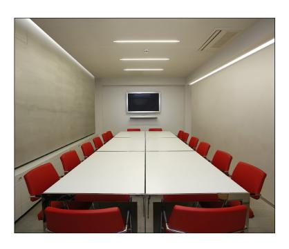
JAKE LED Perimeter is a 3" deep regressed or flush lens style recessed linear luminaire comprised of various apertures, LED light sources and accessory options. JAKE LED 1.65", 2.25", 3.25" and 5.00" can be installed in gypsum ceilings or walls with either a 3/4" Trim (TR) or Trimless (TL) mud-over flange. T-grid for drop ceilings are also available.
