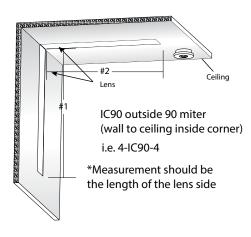
Notes: Drawings are Plan View layout For miters other than 90° contact factory
