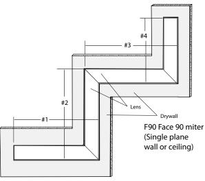
\*Measurement should be the end of miter to end of lens or of the miter (or end of fixture) on the lens slide
