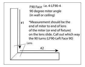
Miter callout key: IC90 - Inside corner 90 OC90 - Outside Corner 90 RF90 - Right Face 90 LF90 - Left Face 90
